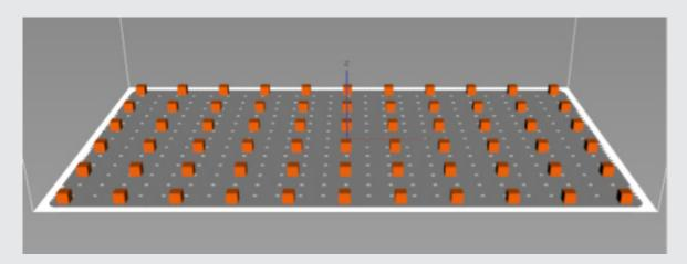
When printing a full platform of aligner dental models with Magna and scanning each model, 90% of the scanned data aligns within +/- 100µm compared to the CAD data, irrespective of the model's position on the platform.
