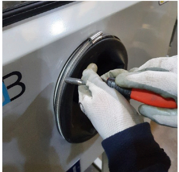
6- Make sure the jubilee clip is pushed back over the ring under the gauntlet
