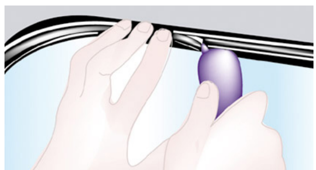
12- The spur on the handle compresses the overlapping filter strip into the channel ensuring a tight joint seal
