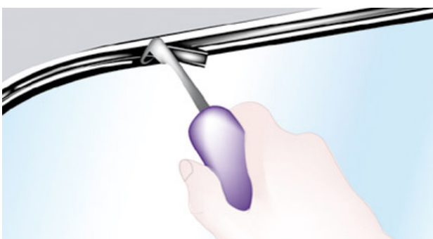
11- After making the complete loop the tool is removed, and the trim bead should be cut to length allowing a 2 or 3mm overlap so it is compressed when in place
