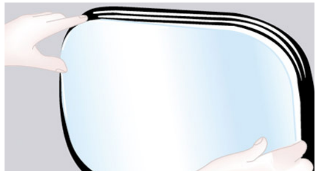
4- Drop the replacement window into the bottom corner first at a slight angle and proceed as far a possible without force
