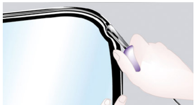
10- The tool slides in the channel all the time feeding the filter strip through the handle and eye. Move/twist the tool slightly from left to right will assist the process
