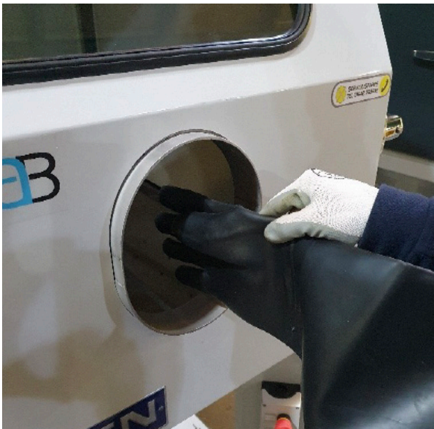
1- Check gauntlet hand position and insert into cabinet
