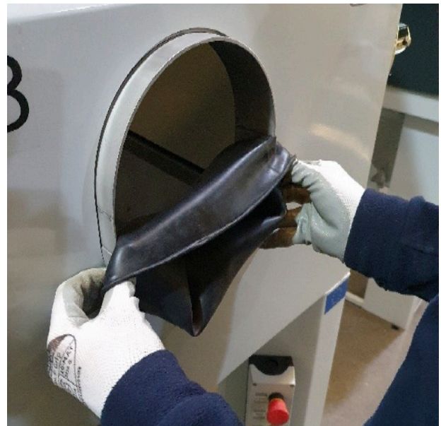
2- Pull gauntlet up and around armhole starting from the bottom
