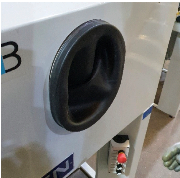
3- Make sure the gauntlet is even and pushed right up over the armhole ring
