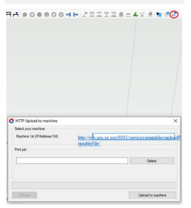
The HTTP Protocol can be set up in the machine workflow properties tab.
