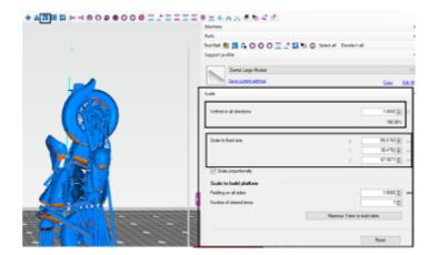
**Tip:** When you apply a scale factor, it will be applied to the part automatically once a value is defined.
