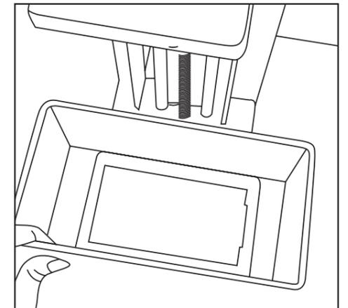
Ensure the base of the vat film is clean. Wearing gloves wipe the bottom of the vat film with a piece of absorbent paper. You can use soapy water or IPA to help cleaning. Make sure the print platform is clean by scrubbing with liquid soap and water and wipe dry. Place the platform on the print arm.
