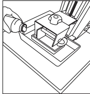
**NOTE:** If you have an object that is 100 cm<sup>3</sup> then it will use 115g of resin. Always overfill by at least 20% to ensure consistent resin flow. For most prints, filling the vat to 1/3 full is more than enough. Place the hood back on the printer.
