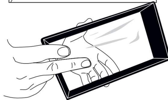
The vat should be tensioned, this can be checked by gently tapping on the film with your finger. not your fingernail!
