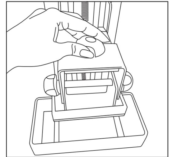
Tighten the upper bolt and loosen the two side bolts on the print platform.
