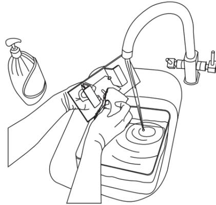
2. Empty and clean the vat after every print. Be sure to clean it thoroughly as any solid pieces on the bottom of the vat would prevent the platform from homing correctly. Pour the resin back into the bottle through the funnel, using the strainer provided.
