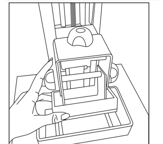
Wearing gloves, press down hard in the middle of the metal platform and then tighten the two side bolts. Press '+10', and the platform will lift 10mm, pour the amount of resin you need, then press '-10' to return it to screen height and you are homed!
