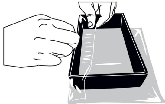
5. Pull each side of the film up and onto the sides of the vat.
