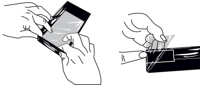
6. Apply single sided tape at the corners over the folds to keep the film tight. The vat should now be tensioned. Trim excess edges off.
