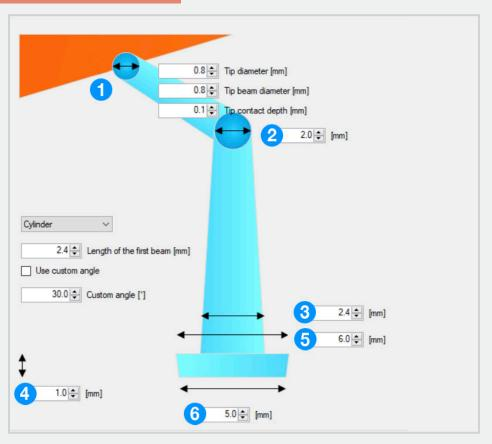
These are recommended support settings in relation to a UV LCD printer with  $81 \mu m$  XY resolution.
