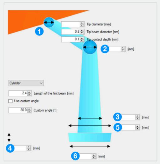
These are recommended support settings in relation to a UV LCD printer with  $81\mu m$  XY resolution.
