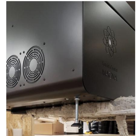
Figure 6: Making sure forks reach fully under the printer before lifting
