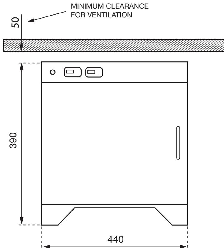
Figure 2: Cure M+ space requirements, front view
