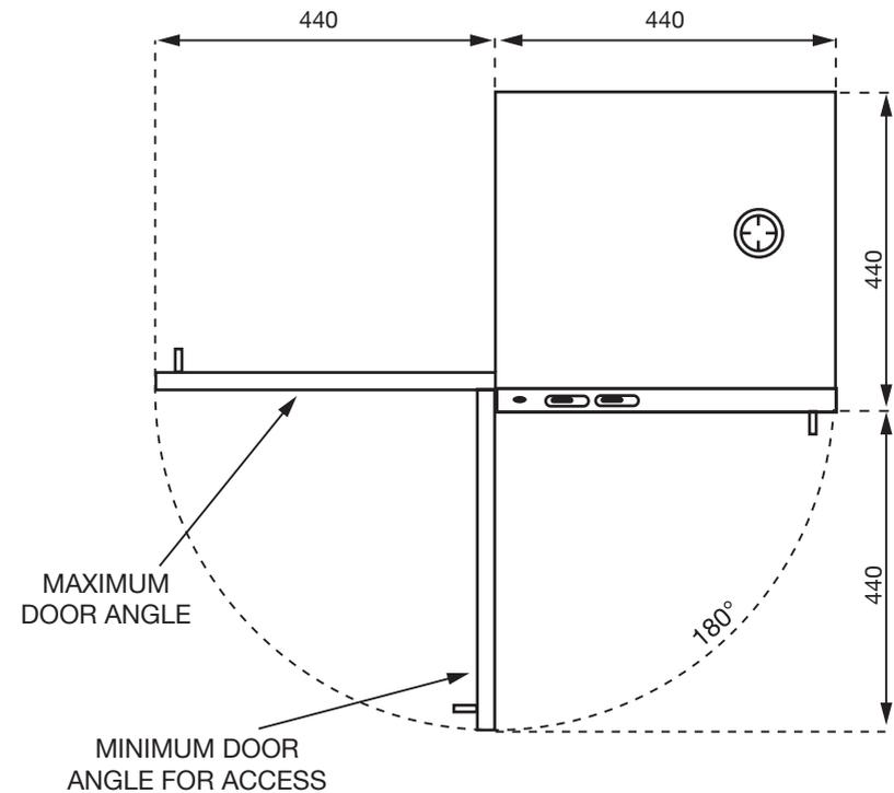
Figure 3: Cure M+ space requirements, plan view
